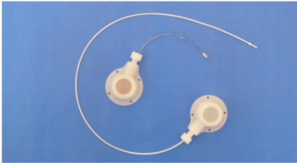
**The Jet Port Allround Catheter** consists of an ultra thin silicone catheter with an inner diameter of 0.6 mm and external diameter of 1.05 mm which is connected with a screw connector to the port chamber. Behind the tip of the catheter, there is an olive rim for end-to-side fixation in the artery (Fig. 1).
